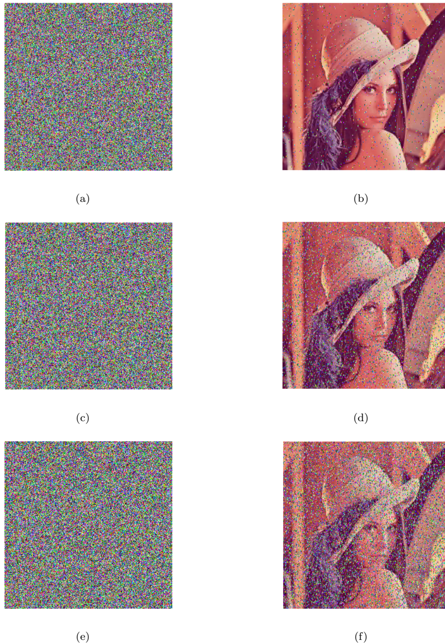
FIGURE 5.8: Experimental results for the performance evaluation of data loss attacks: (a, c, e) cipher images with 1%, 5% and 10% salt and pepper noise, (b, d, f) decryption results of corresponding images using our scheme.
